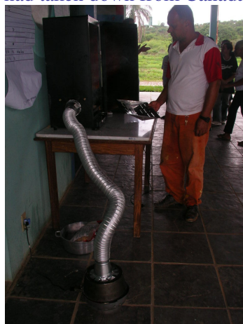
15. The automated smoke generator was adapted to local conditions using a pan of woodchips placed over an electric heating element.
