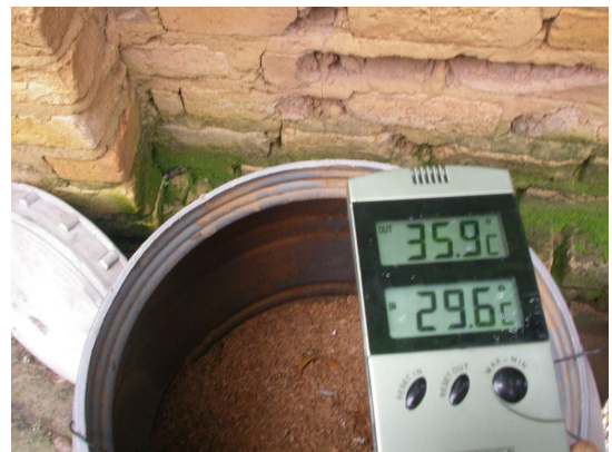
10. Within two days the inner temperature increased 6°C
