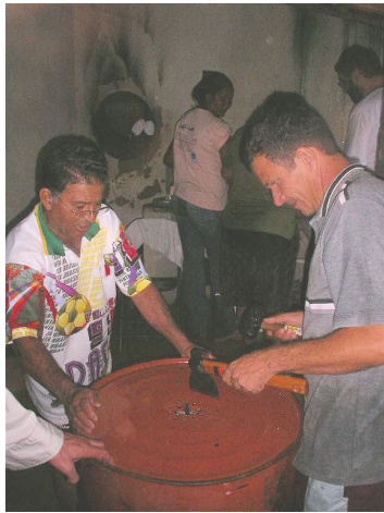
27. Josémar Alves implements his plans to transform an steel drum into a smoker
