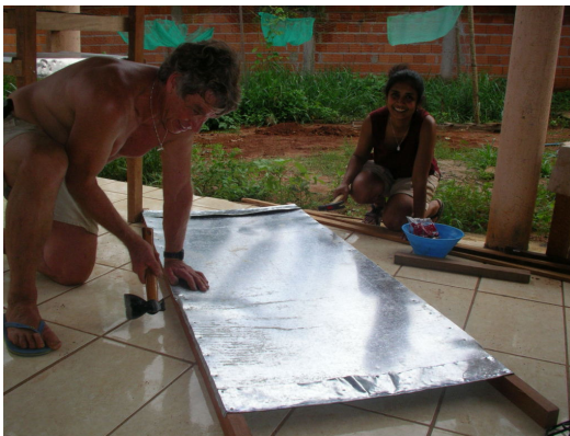
3. Attaching sheet metal to base frame of solar chamber
