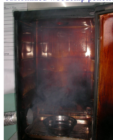
16. The smoke generated was piped into the Bradley smoker unit using an air duct.
