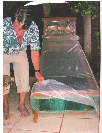
8. The air intake is protected by mosquito netting from entry of insects
