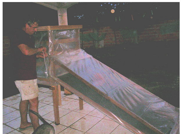
10. Only two bolts connect the solar chamber and the drying chamber
