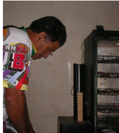
14. The Bradley smoker is fitted with an automatic smoke generator, which uses customized woodchip pellets.
