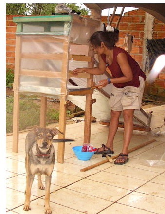
6. Assembly of drying racks. A “door” access is simply a weighted plastic sheet
