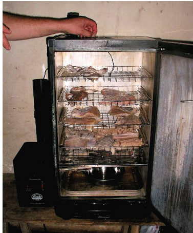
13. The fish are then loaded into the semi automated Bradley smoker that the WFT team had taken down from Canada
