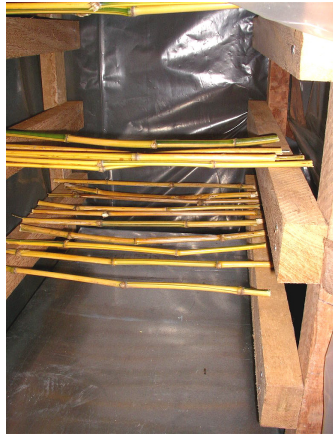
7. Drying racks can be made of stainless steel or a wood that can be hygienically cleaned
