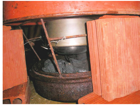
34. A truck wheel rim is used to hold the charcoal to generate heat and smoke
